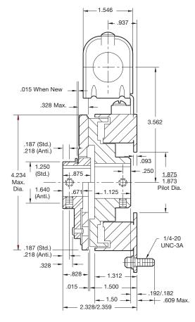
\*Mounting holes are within .010 of true position relative to pilot diameter.
