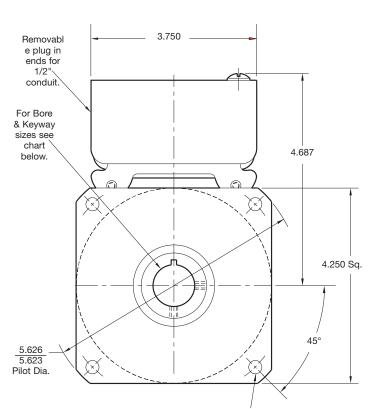
.296/.280 dia. (4) holes equally spaced on 5.000 dia.\*
