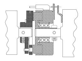
SFC Clutch Coupling Typical Installation
